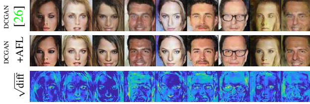
Figure 2: Contribution of AFL: Face generation results of (top) DCGAN [26] and (middle) integrating DCGAN within the proposed AFL framework. Faces generated by DCGAN+AFL are sharper and show fewer artifacts. (bottom) The differences between the images generated without and with AFL highlight that AFL corrects the spatial regions that suffer from artifacts, for example, the cheek of the left-most face, and the eyes of the second from left.
