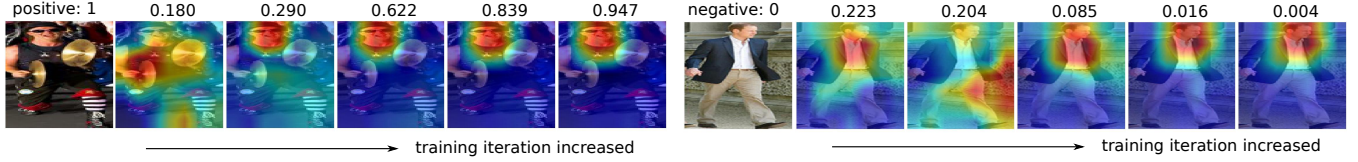
Figure 2. Attention heatmaps for label “sunglasses” in different iterations of CNN (ResNet50) model training, where face is the desired label-relevant region. The number above each attention heatmap represents the predicted presence score (in [0, 1] ) in the corresponding iteration.
